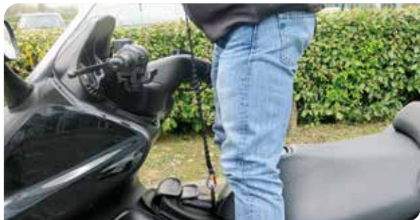
PHOTO NO. 13 : VEHICLE STRAP LENGTH ADJUSTMENT ON A SCOOTER
