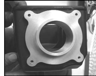
15. Install the provided adapter into the air box. Make sure the holes line up.
